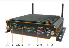
A: SMA Antenna B: DC Power Input
