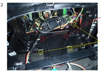
Position the clamp mounts (two pieces) and put the bracket in place. *Note* the fastening points (2) for the clamp mounts.
