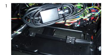
Dismantle and remove the instrument panel in the center to lay off the top frame of the dashboard center.
