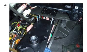
Attach the extension bracket in Zirkona Dashboard Mount with spacers.
