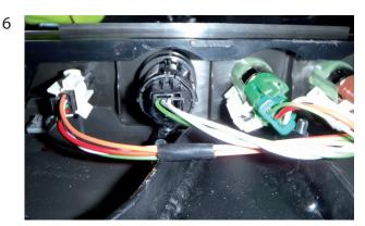
It is important to protect the cables so that they do not rub against the bracket.
