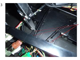
Make a mark in the plastic for spacers (4 holes). The spacers must pass through the plastic to secure the bracket which extends the mount and makes it visible for final assembly.
