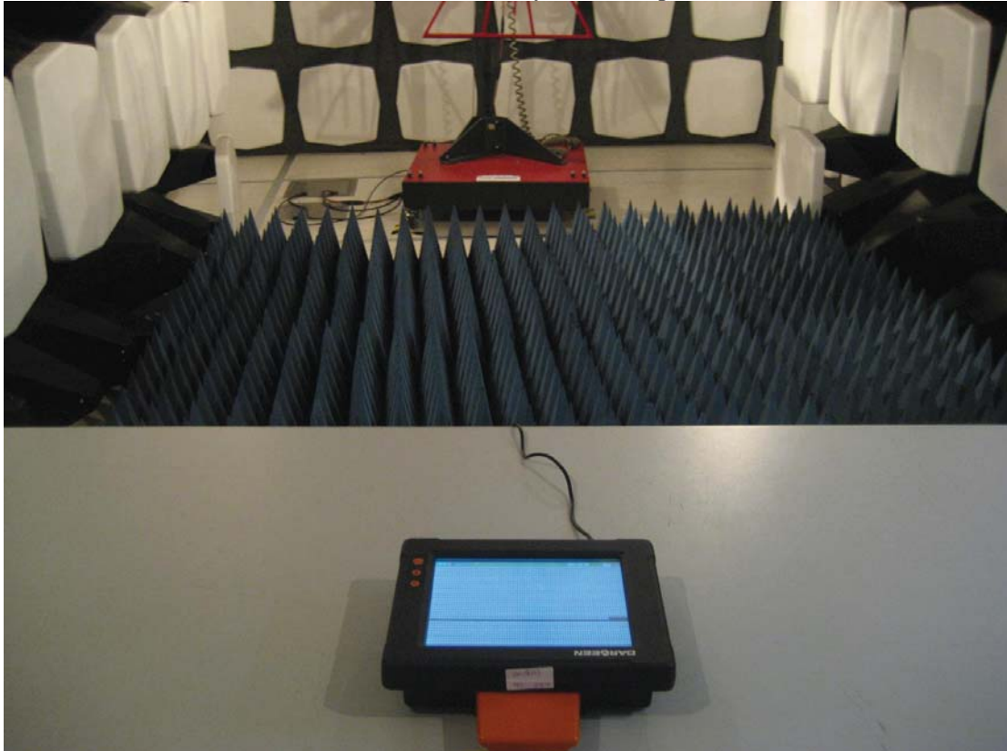
Radiated Immunity Test Set Up
