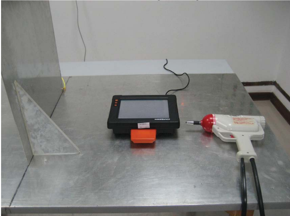
Electro Static Discharge Test Set Up
